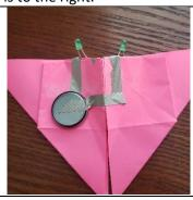
Wire the negative LED by attaching a piece of maker tape to the negative lead of the left LED and around to the back of the butterfly. Folding carefully, direct the tape to the negative side of the battery, being sure not to cross over any of the positive circuitry.
