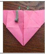
Wire the positive LED by attaching a piece of maker tape to the positive lead of the right LED and wrapping it around to the back of the butterfly. Fold a piece of tape into a loop with the sticky side facing out. Place that on the tape you added to the back.
