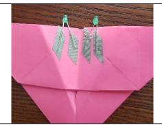
Lay the butterfly flat. With the positive lead (the longer one) to the left, tape one LED to the left side of the butterfly. Use the maker tape on each lead, making sure that the positive and negative ends do not touch. Tape the right LED down in the same way, this time ensuring that the positive lead is to the right.
