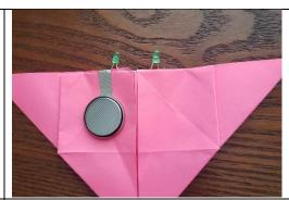
Use the sticky loop of tape to attach the watch battery to the circuit, positive side down.
