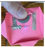
Place the battery under one of the corner folds with the positive side lined up with positive marker and the negative side lined up with the negative marker.
