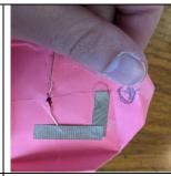
Tape the short end of the LED to the negative line. Place tape strips along the lines you drew connecting the short end to the negative circle you drew.
