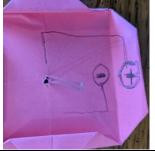
Draw a line from the negative circle to one side of the LED and a line from the positive circle to the opposite side of the LED.
