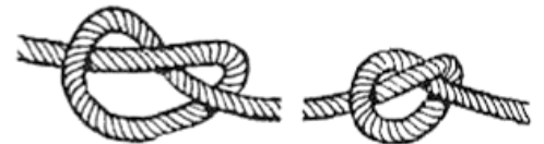
Overhand Knot. Source: commons.wikimedia.org/wiki/File:Boys%27_Life,_1_-_Overhand_Knots.png
